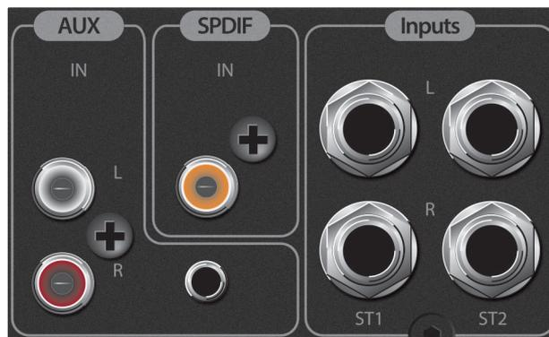
**ST1 L/R:** Connect the left and right channels of your primary stereo source to these balanced 1/4" TRS jacks.
