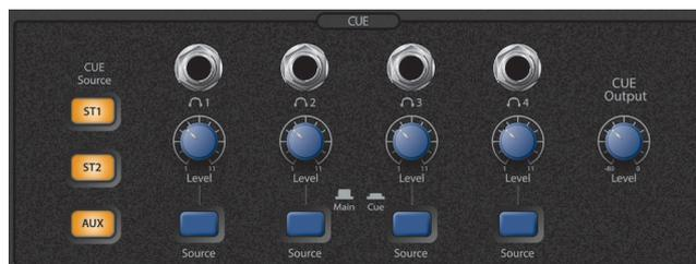
The Cue section of the front panel allows you to manage the Monitor Station V2's Cue system and control its four individually controllable headphone outputs. Each output has its own input selector and its own volume control.
