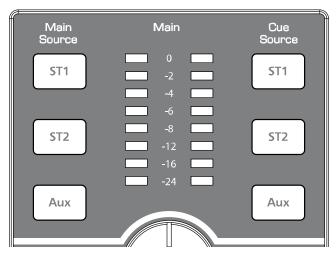
• <u>Main Source</u>. Sets the Main bus' input sources. The Main bus is the source for the Speaker outputs, Main L/R outputs and any headphone amplifiers whose source is set to 'Main'.
