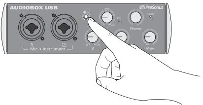
1. Turn up the Channel 1 level on the AudioBox USB while speaking into the microphone. You should see the input meter in Studio One Artist react to the input. If you do not see input metering, verify that your track is armed for recording.
