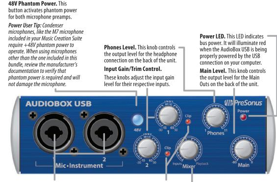
**Microphone / Instrument Inputs.** Each input channel has both a microphone and an instrument preamplifier. The combo connectors allow you to use either a 14" TS or the included XLR cables. Use the 14" connection for guitars and other unamplified instruments. Use the XLR connections to connect your M7 microphone. **Clip Indicator.** Both channels feature a clip LED next to each trim control. This light will illuminate red when the channel's input signal reaches 0 dBFS.
