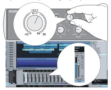
2. Adjust the gain so the input level is near its maximum without clipping (distorting).
