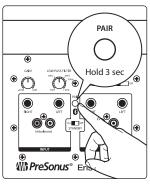
Your Eris Sub 8BT can be paired with any Bluetooth device for audio playback. To pair your subwoofer, first press and hold the pair button on the rear of the subwoofer for three seconds.
