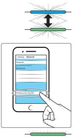
The Power/Bluetooth LED on the front of the active speaker will flash blue and green, indicating pairing is active.
