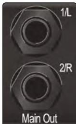
**Main Outs.** These are the Main outputs for the Studio-series interface. The output level of the Main outputs is controlled by the Main level control on the front of the unit. Playback streams 1 and 2 are routed to these outputs.
