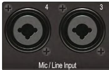
**Mic/Line Inputs (Studio 68c).** These mic/line combo connectors are for use with microphones on the XLR input and with line-level devices via the 1/4-inch TRS connections.
