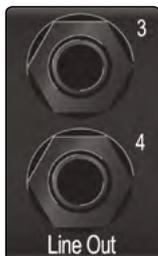
**Line Outputs.** These 1/4-inch, balanced line outputs allow you to route to external devices, such as headphone amps, signal processors, and additional monitors. Each output has an independent playback stream (Playback streams 3 and 4).
