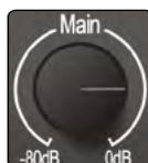
**Main.** The main knob controls the output level for the main left/right outputs on the back of your Studio-series interface and has a range of -80 dB to 0 dB. This control provides attenuation only.
