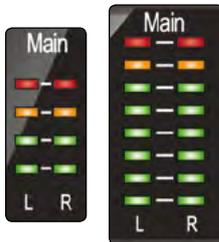
**Output Meters.** These meters display the signal level received from the first two driver returns (Main Left/Right). These meters have the same range as the input meters and display the signal level before the main output level control.
