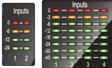
**Input Meters.** These LED meters show the input level of the analog inputs on your Studio-series interface. The red Clip LED will illuminate when your input signal reaches -0.5 dBFS. At this level, the signal will begin to overload the analog-to-digital converters and exhibit signs of clipping. Use the gain controls to keep the signal below this level.
