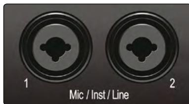
**Microphone Inputs.** Your Studio-series interface is equipped with high-quality microphone preamplifiers for use with all types of microphones. The Studio 26c features XMAX-L solid-state microphone preamps that are optimized for bus powering. The Studio 68c features XMAX microphone preamps with a Class A input buffer, followed by a dual-servo gain stage.
