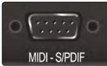
**MIDI and S/PDIF Breakout-Cable Connector (Studio 68c).** This is where you connect the breakout cable for the MIDI and S/PDIF I/O.
