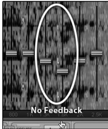
You can apply this process to the Main system, as well. This is especially useful with applications requiring lavalier or podium mics. These types of microphones are typically omnidirectional condensers and are very prone to feedback.
