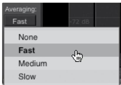
While the RTA is engaged, you can adjust its averaging speed. When using music in test measurements, it is often necessary to average the data over a brief amount of time. This is because most musical signals do not have energy at all frequencies all of the time.
