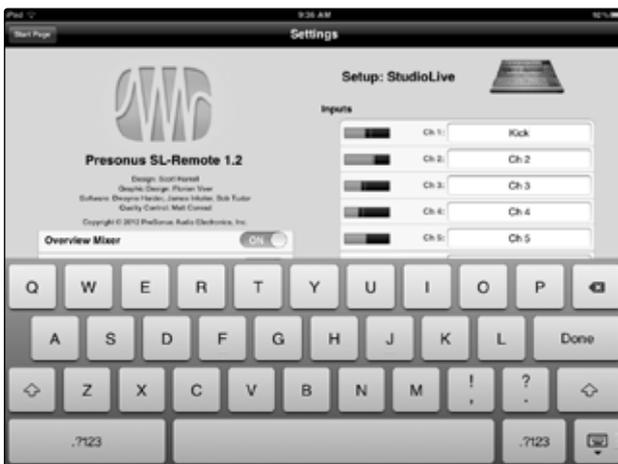
To create a custom name for any channel, aux, or subgroup in your mix, simply tap on the text field next to it. This will launch the iPad keyboard. After you have entered the new name, tap the Done button. The channels' default name will be replaced with its new custom name in SL Remote, VSL, and QMix.
