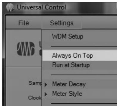
When this is enabled, the Launch window will remain in the foreground when other applications are active, rather than being in the background behind the current application's window.
