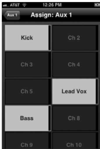
Once you've identified these channels as your "Me" channels, the Wheel of Me will increase or decrease the level of these channels concurrently, allowing you to create a subgroup of your most critical channels in your monitor mix.
