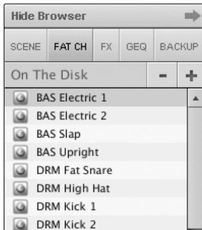
To load every component in a Fat Channel preset (gate, compressor, EQ, etc.), select the preset from the Browser window and drag it over any part of the desired channel. If you drag it over any of the component Quick Views, it will load only that component (e.g., if you drag a preset over the gate Quick View, only the gate will be loaded).
