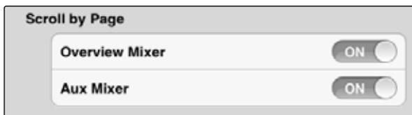
When the Scroll by Page option is enabled, the mixer will scroll to through channels by entire pages, rather than by individual channels. Turning this option off will allow you to scroll over by a single channel and offer more granular control.
