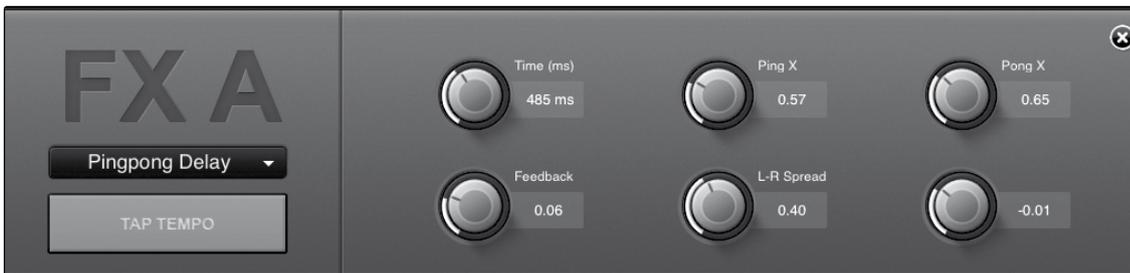
To load a new effect type, tap on the Effects Type window, and then tap on the new effect type to load it. To adjust a parameter, simply tap on it and move your finger up or down while maintaining constant contact with your iPad.
