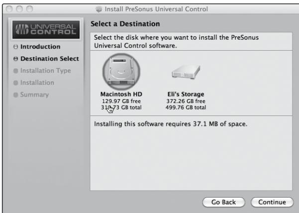
2. You will be directed to choose the hard drive onto which you want to install the StudioLive driver and Universal Control with VSL. You must choose your system drive. Storage drives and partitions cannot be used as hosts for the driver.
