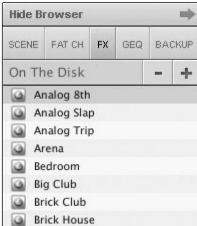
To load an FX preset, select it from the Browser window and drag it over any part of the desired FX bus in the Master section of the Overview tab. Once it is loaded, you can use the FX Type menu to change the effect and create new presets.
