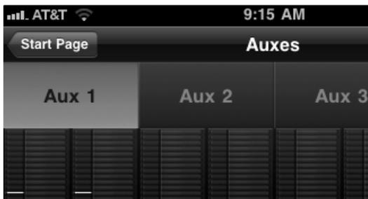
To create an Aux Mix using StudioLive Remote, tap on the Aux Mix Select tab for that Aux. The selected Aux Mix tab will be highlighted to alert you that its individual channel send levels will be displayed below.
