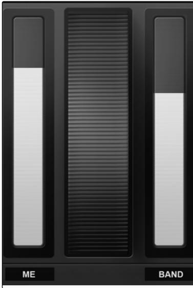
The Wheel of Me increases or decreases the level of your Me Channels as a mix relative to the rest of the channels. If you increase the level of your Me Channels beyond the top level, the rest of the channels will decrease in volume.
