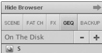
To load a graphic EQ preset, select it from the Browser window and drag it over any part of the focused graphic EQ. Graphic EQ presets can be loaded on the Overview tab or the GEQ tab. Once a preset is loaded, you can use the sliders in VSL, or the encoders on the StudioLive, to make adjustments. Note that you must be in the GEQ menu page for the graphic EQ you wish to control in order to use the encoders on your StudioLive to control each graphic EQ in VSL. See the next section for details.
