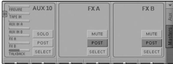
The Masters view displays the controls for each aux output and FX bus as they appear on the StudioLive and displays a scribble strip to give each aux a custom name.
