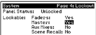
4. To lock your StudioLive, press the System button in the Digital Effects | Master Control section and navigate to Page 5: Lockout. Your StudioLive cannot be locked unless this page is active. If you have two StudioLive mixers linked, you only need to lock the Master unit to lock both mixers in the chain.
