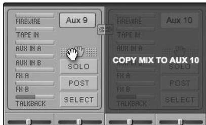
Next to the main fader, and in each of the aux masters, you will see the Copy Mix handle. When clicked on, this handle lets you drag-and-drop the mix for that bus to another bus. In this way, you can drag the main-fader mix to Aux 1 to set a starting point and can quickly give the singer the same mix on two different floor wedges.
