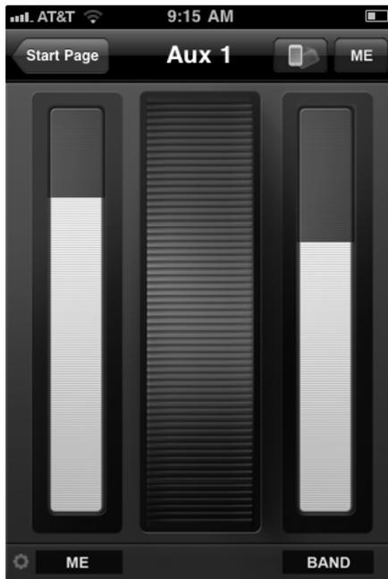
QMix's Wheel of Me provides you with an easy and powerful way to control all of the channels that contain your voice and instruments. To open the Wheel of Me, turn your iPhone/iPod touch to the Portrait view. The Wheel of Me will open for the currently selected aux mix (so if you have Aux Mix 3 selected on the Aux Mix page, Aux Mix 3 will still be selected when you open the Wheel of Me).
