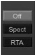
By default, Smart analysis is disabled. While Smart is disabled, you have control over which bus is routed to Auxiliary Inputs 29 and 30 (StudioLive 16.4.2 and 24.4.2).
